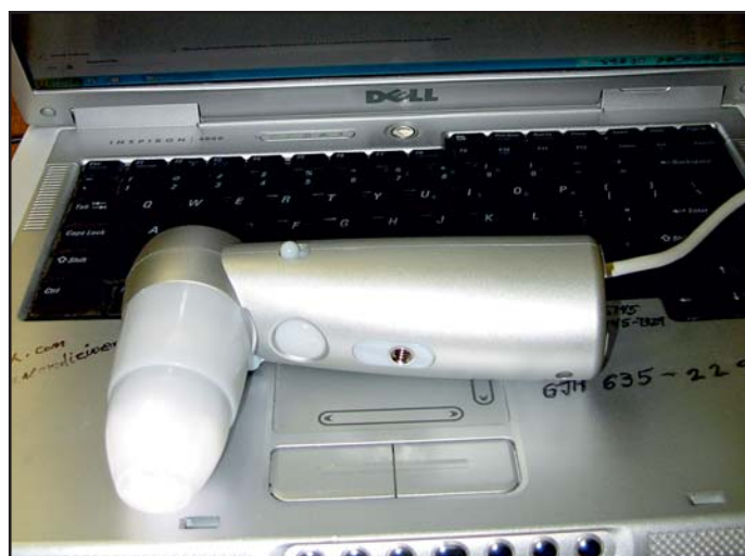
Fig 2. Using a 50x magnification USB microscope (MDS – Medical Diagnostic Services, www.mdsincorporated.com ), the bird was examined. This portable microscope is a valuable tool that captures images directly onto the computer for close observation by and discussion with the client. Still images can be saved for future reference.
