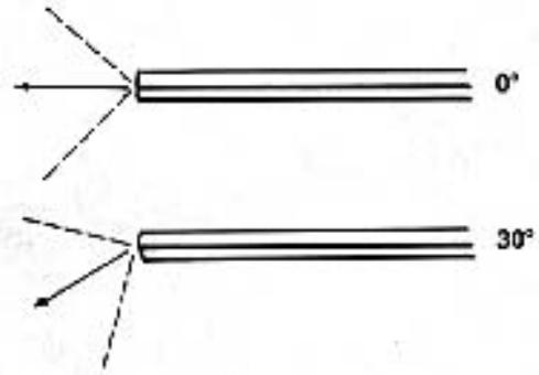
**FIG 13.5** Endoscope lens with a 30° offset allows for improved vision in confined spaces.
